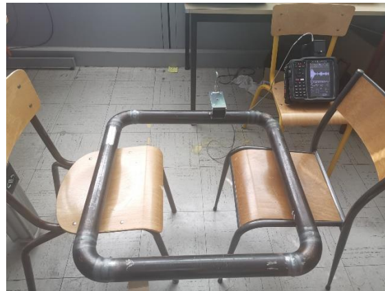
Figure 2: Experimental setup with a carbon steel pipe loop with elbows and defects.
